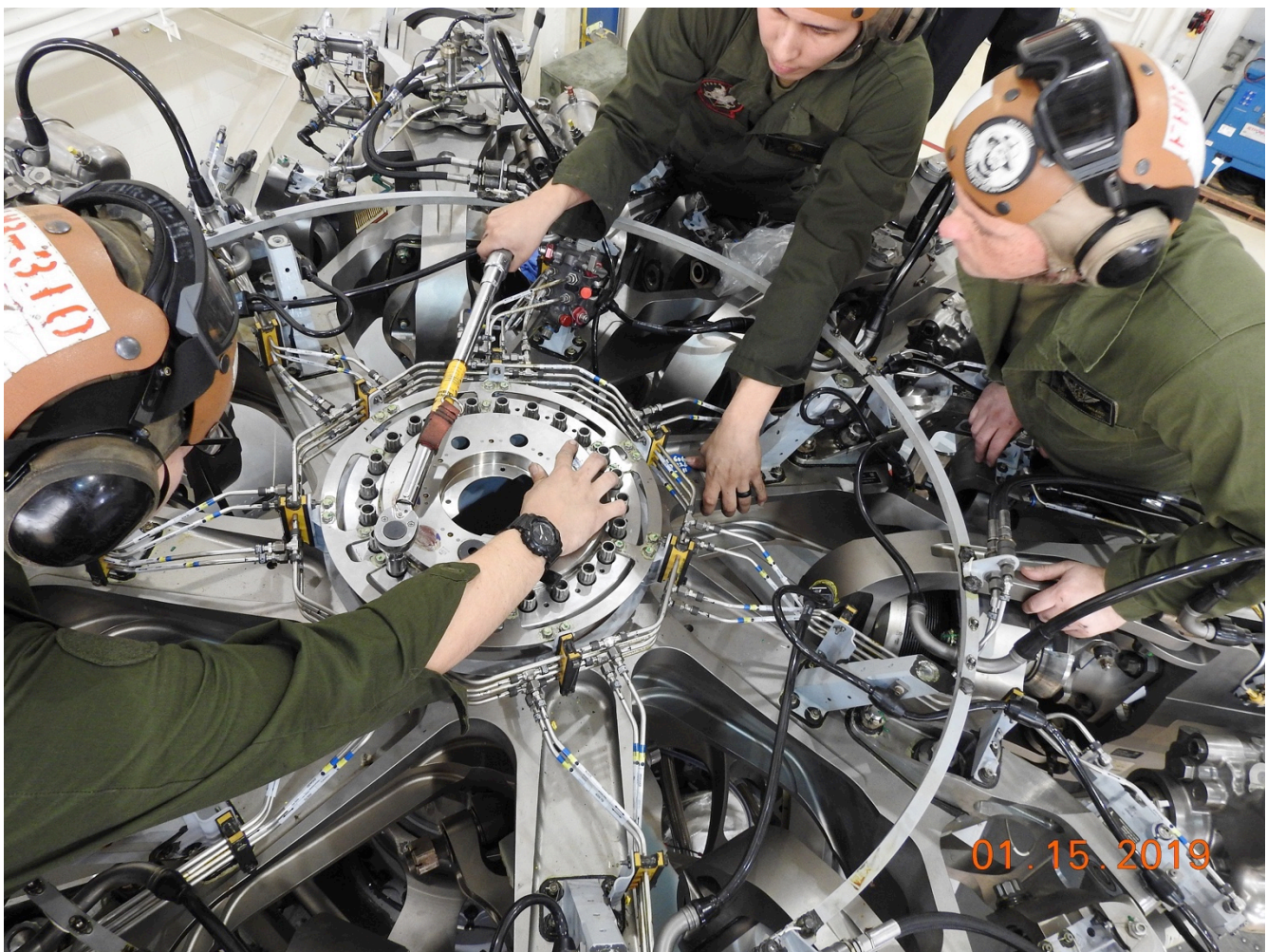
Figure 5 Marines working on the rotor head which is a major piece of what allows the aircraft to carry three times the weight externally compared to a CH-53E. VMX-1
