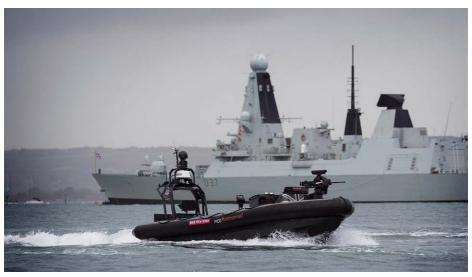
An experimental trial is completed in 2019 with a BAE Systems' unmanned surface vessel, fitted with lightweight remote surface weapon. The vessel can operate for up to 10 days at 'patrol speed' or 300 nautical miles in pursuit mode, reaching speeds of up to 45 knot.
