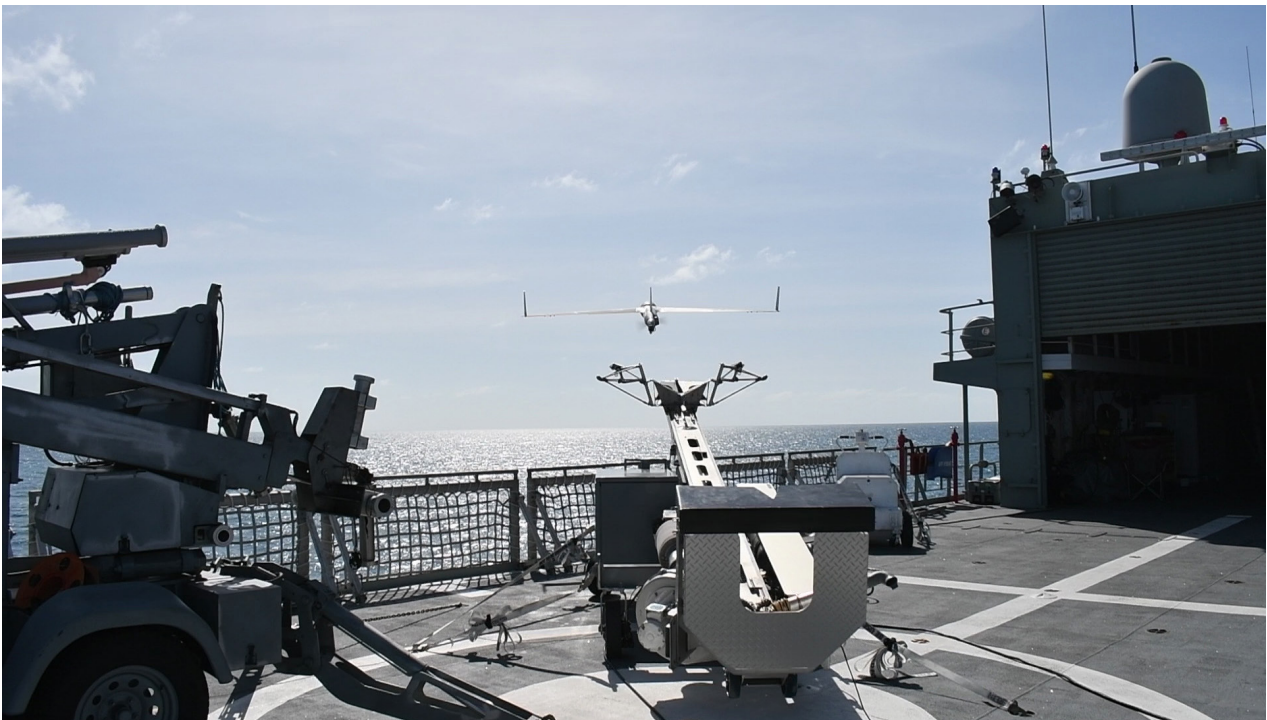
Figure 1: 822X Squadron launches a ScanEagle from HMAS Leeuwin at sea
