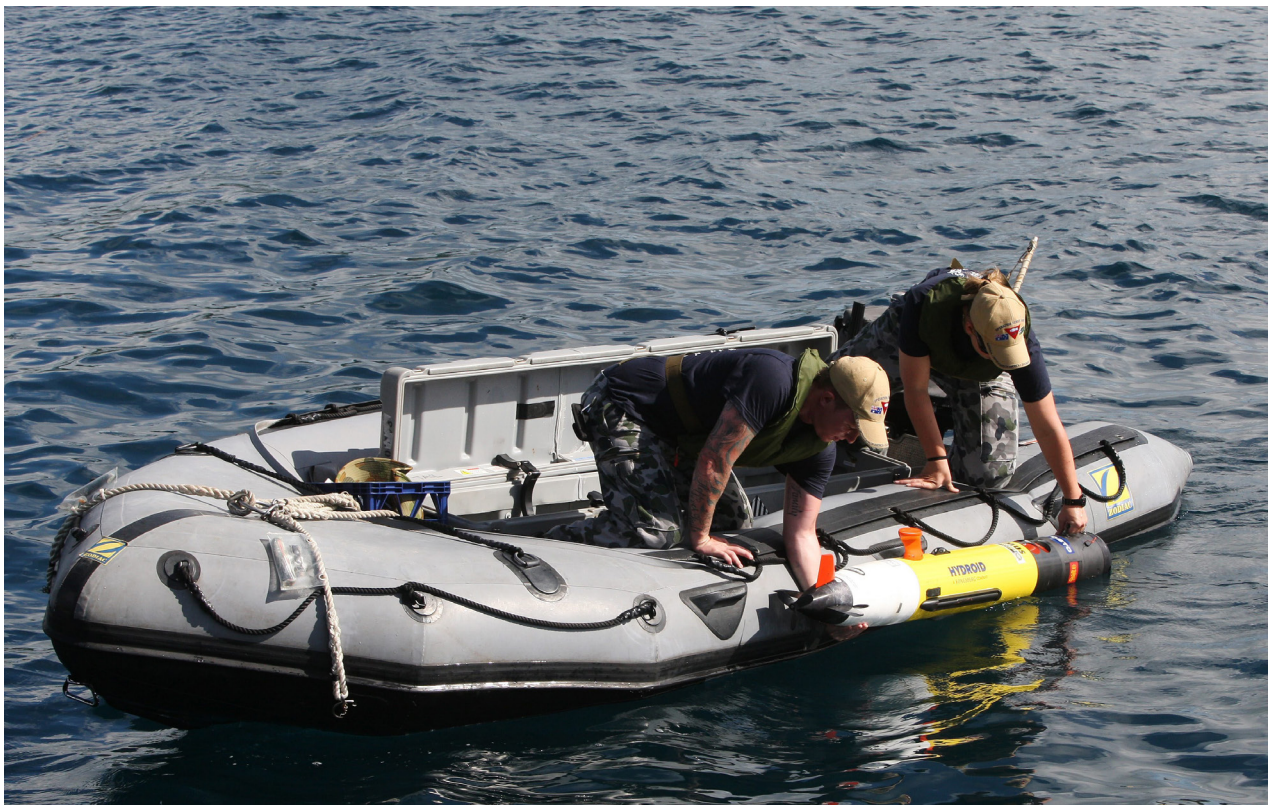
Figure 2: Navy personnel launch the REMUS, an autonomous underwater vehicle for locating ordnance on the seabed, off Talaghi Island as part of Operation Render Safe 2013
