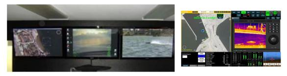
The single supervisory control station for the three LUSVs remains manned in the mothership for the initial transit to the MUSV departure point, at which time, two others will be manned to provide further supervisory control.
