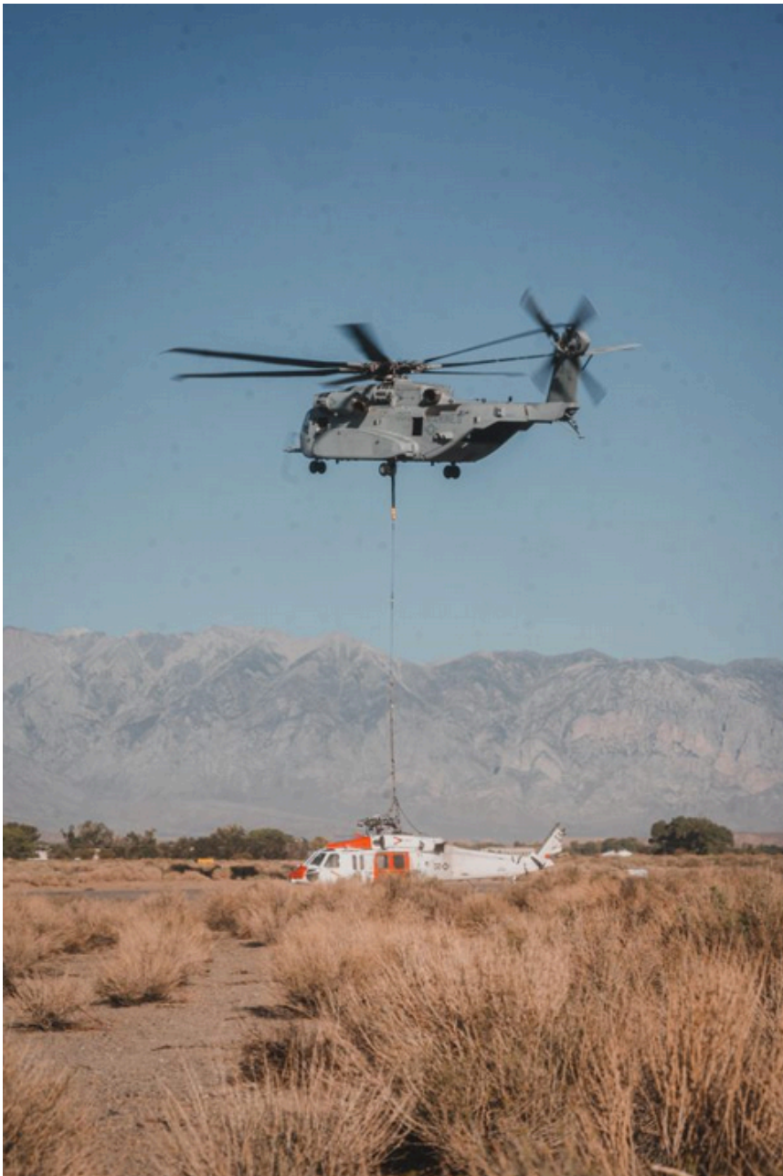
A Marine Corps CH-53K King Stallion lowers a Navy MH-60S Knighthawk helicopter to the ground after recovering it from the nearby mountain ranges after it conducted a hard landing near, Bishop, California, Sept. 5, 2021. The two-day operation was the first official fleet mission for the CH-53K King Stallion, as it is currently undergoing an operational assessment while the Marine Corps modernizes and prepares to respond globally to emerging crises or contingencies. (U.S. Marine Corps photo by Lance Cpl. Colton Brownlee)
