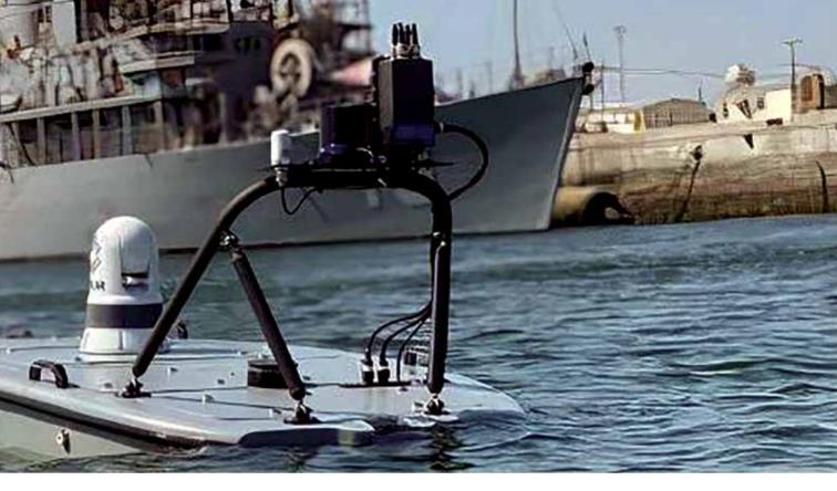
was one of the highlights of this month-long event. The catamaran-hulled MANTAS was able to operate in sea state five conditions. Additionally, the USV has a number of compartments that protected sensor components in heavy weather.
