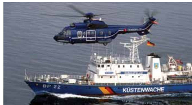
Nearly 70 percent of the Super Puma fleet is operated in offshore transport. Large sliding doors allow for the transportation of bulky freight and rear access enables large loads. It is widely used by firefighters, police and emergency services. Photo credit: EADS
