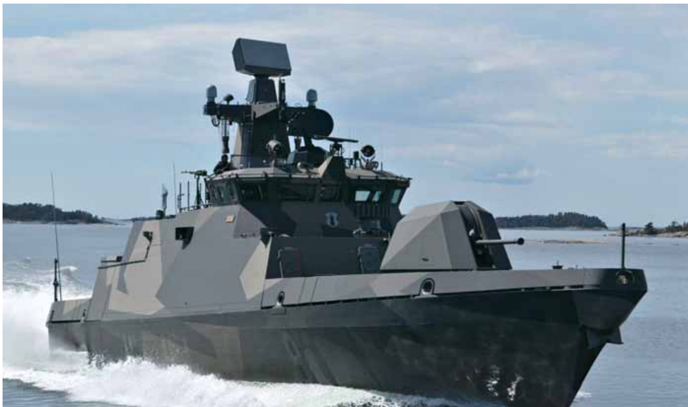
The multimode radar system TRS-3D – pictured here on a Danish Stanflex 300-class ship — is specially suited for deployment in littoral waters and has been deployed successfully on several types of naval ships worldwide. Photo credit: Cassidian
