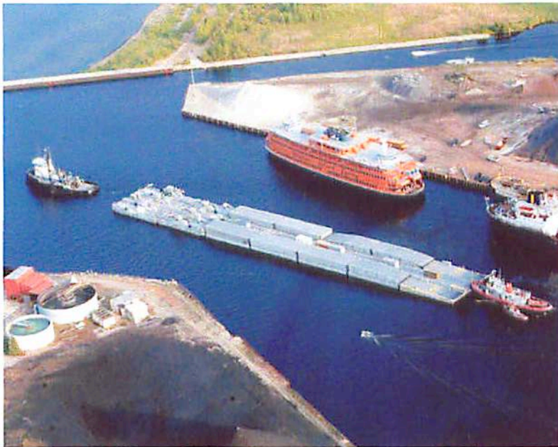
For the Sea base to work as well as is desired, new technologies will be needed to facilitate operations such as trans-shipping of equipment and materiel. Here, the US Navy's Improved Modular Lighterage System is tested.
