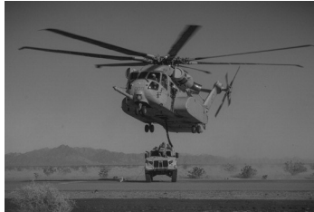
A U.S. Marine Corps CH-53K King Stallion helicopter, assigned to Marine Aviation Weapons and Tactics Squadron One, executes an external lift of a High Mobility Multipurpose Wheeled Vehicle during Weapons and Tactics Instructor (U.S. Marine Corps photo by Lance Cpl. Elizabeth Gallagher)
